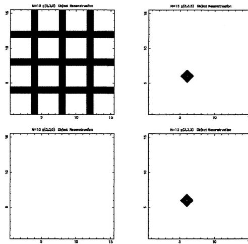
Figure 7: The top left image shows the basis function reconstruction of the intensity at the input plane and the top right image shows a contour map of the coherence function of the array at the same plane centred on a single pixel. Each bolometer element is made up of 9 mutually incoherent pixels and each element is also mutually incoherent. The bottom left plot shows the intensity at the Fourier plane and the bottom right the coherence function at the same plane centred on a single pixel.
