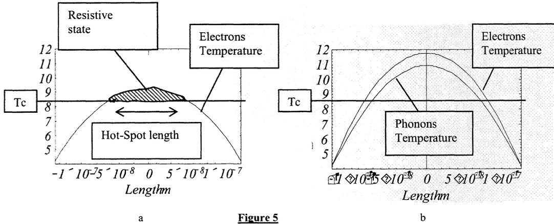
It is clearly shown in fig.5 that the minimization of the substrate, which usually acts as an energy acceptance reservoir, now increase the electron temperature profile of the film. In clear, the phonon will heat up the electron in the film. Indeed, the superconducting nanobridge will need less microwave power irradiation to be driven into the resistive state. Then, the sensitivity of the membrane-based HEB mixer should be higher.
