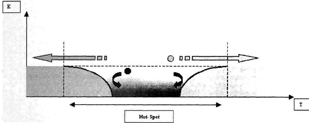
**Figure 1:** Schematic of a HEB bridge. The whole bridge is heated by RF, the bias heating acts only on the hot spot where superconductivity is suppressed. The electrons are cooled by phonon escape to the substrate and by outdiffusion to the pads. Outdiffusion is reduced by Andreev reflection at the hot spot boundary. We can consider the heat Andreev transmission coefficient as:
