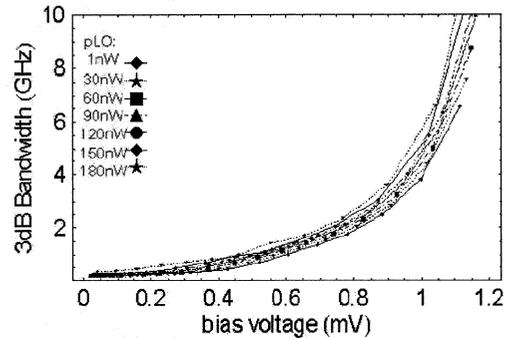
Figure 4: IF bandwidth versus bias voltage curves.
