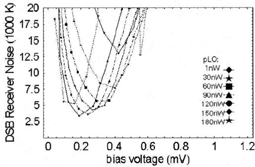
Figure 3: DSB Receiver Noise Temperature versus bias voltage
