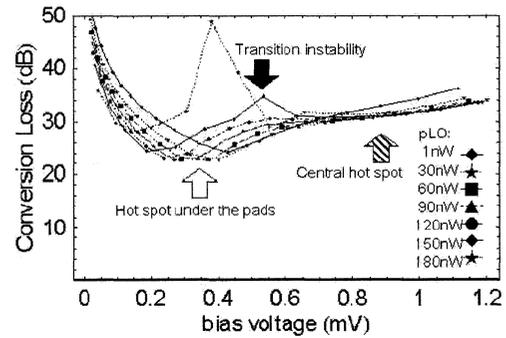
Figure 2: Conversion loss versus bias voltage curves.
