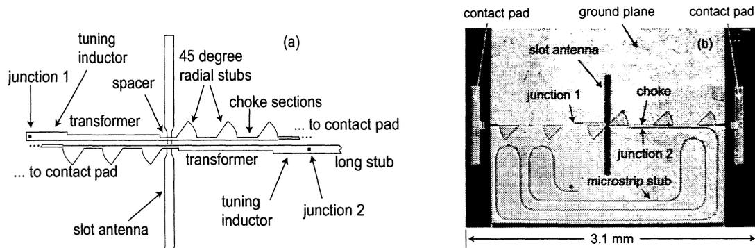
**Figure 1:** (a) Schematic diagram of test device. (b) Photograph of a 100 GHz test device with a 10 mm long microstrip stub. The Nb top strip is 5  $\mu\text{m}$  wide, and 4000  $\text{\AA}$  thick. The thickness of the Nb ground plane layer is 2000  $\text{\AA}$ . The thickness of the SiO dielectric is 4000  $\text{\AA}$ .
