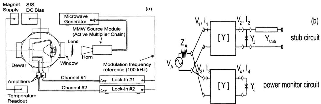
**Figure 2:** (a) Schematic diagram of experimental setup. (b) Equivalent circuit model of the device. The two junctions are connected in parallel to the slot antenna through two identical matching circuits, which we treat as two-port black box linear circuits, characterized by an unknown admittance matrix  $Y$ .
