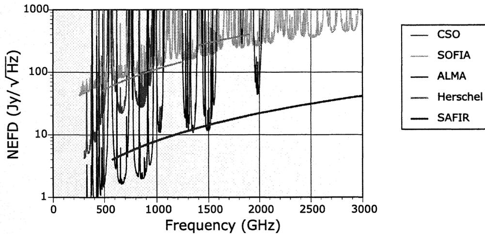
FIGURE 4. Flux density sensitivity at 1km/s resolution from 300 GHz to 3 THz (100 μm to 1 mm) of several facilities envisioned for the coming decade, as compared to the sensitivity of the SAFIR observatory.
