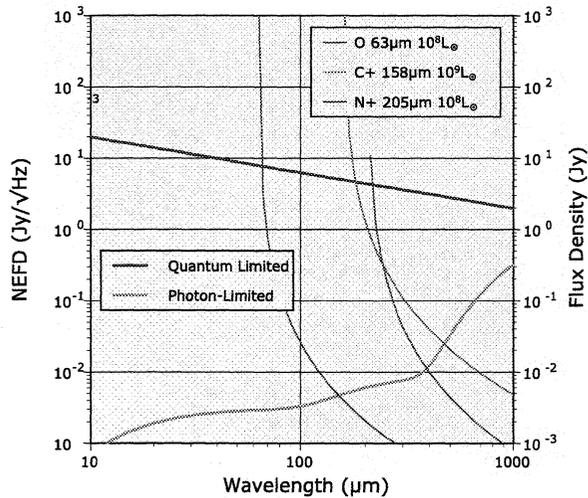
FIGURE 3. NEFD for a  $\lambda/\Delta\lambda=3\cdot 10^5$  (1km/s resolution) spectrometer using photon-limited direct detectors compared with quantum-limited coherent detectors. Predicted fluxes for redshifted fine-structure lines are shown for reference.
