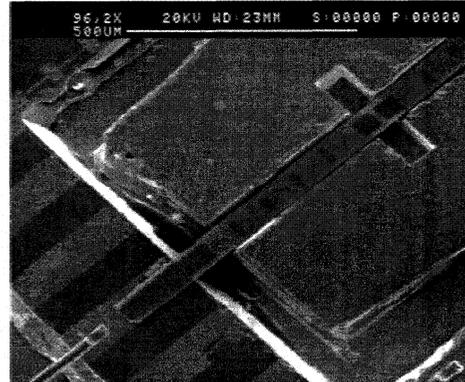
Fig 4. SEM-Picture of suspended membrane into the waveguide
