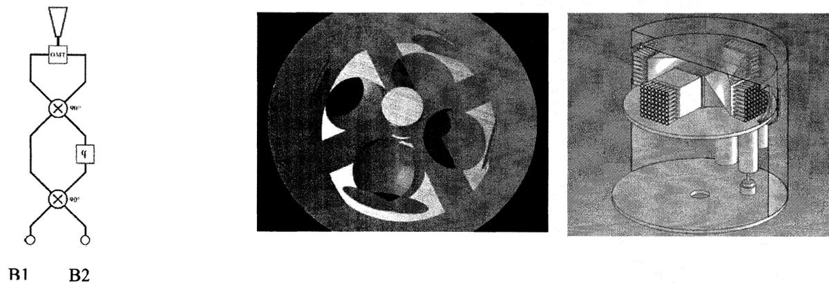
Figure 2: **Left:** Schematic view of the pseudo correlation receiver. **Middle:** A schematic view of a CLOVER telescope with four co-pointing Compact Range Antennas (CRA). Each CRA is fed by 64 horns. **Right:** The central cryostat containing four 64-feed arrays and the sections behind containing the hybrids and phase switches.
