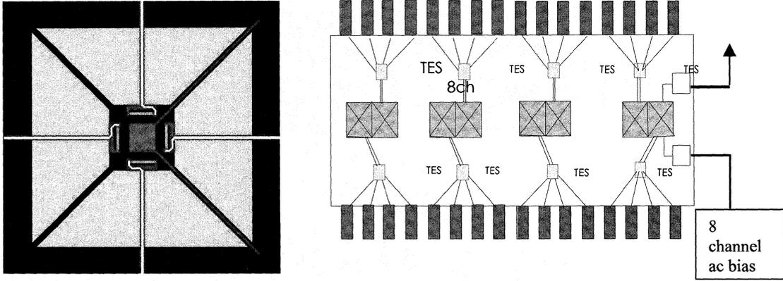
Figure 4: (a) Scale layout of a single pixel with TES (red), Nb bias lines (blue), microstrip line (white on blue) and termination resistors (green). The nitride membrane is removed in the regions shaded yellow. (b) Schematic of a detector module. 32 fin-lines are coupled to 8 TES and a single 8 channel multiplexer. Read-out is by a single wideband, low noise SQUID.
