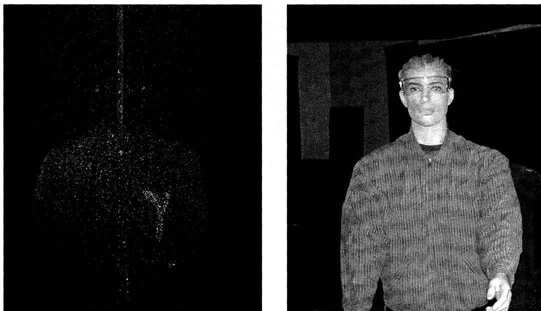
Figure 7. 1.56 THz image of dressed mannequin with concealed weapon (left), photograph of the mannequin as measured (right).
