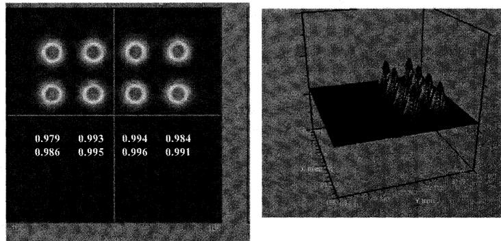
Figure 7: Output Field of 8 pixels at the CFP. The top 8 beams of SEQUOIA are launched from the SEQUOIA focal plane through the RO System, and plotted at the CFP. The coupling efficiencies to the required gaussian beams at the CFP for the 8 pixels are noted in the lower half of the figure. The figure on the right shows the isometric surface plot of the SEQUOIA beams at the CFP.
