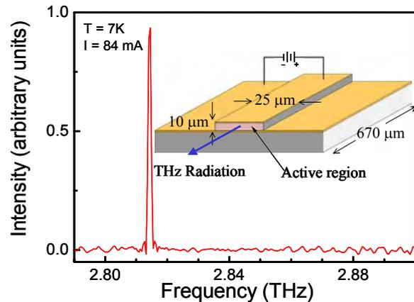
Fig. 1. Emission spectrum of the quantum cascade laser biased with a DC current  $I$  of 84 mA and operated at a temperature  $T$  around 7 K. The inset shows a schematic view of the QCL and the dimensions of the laser cavity.
