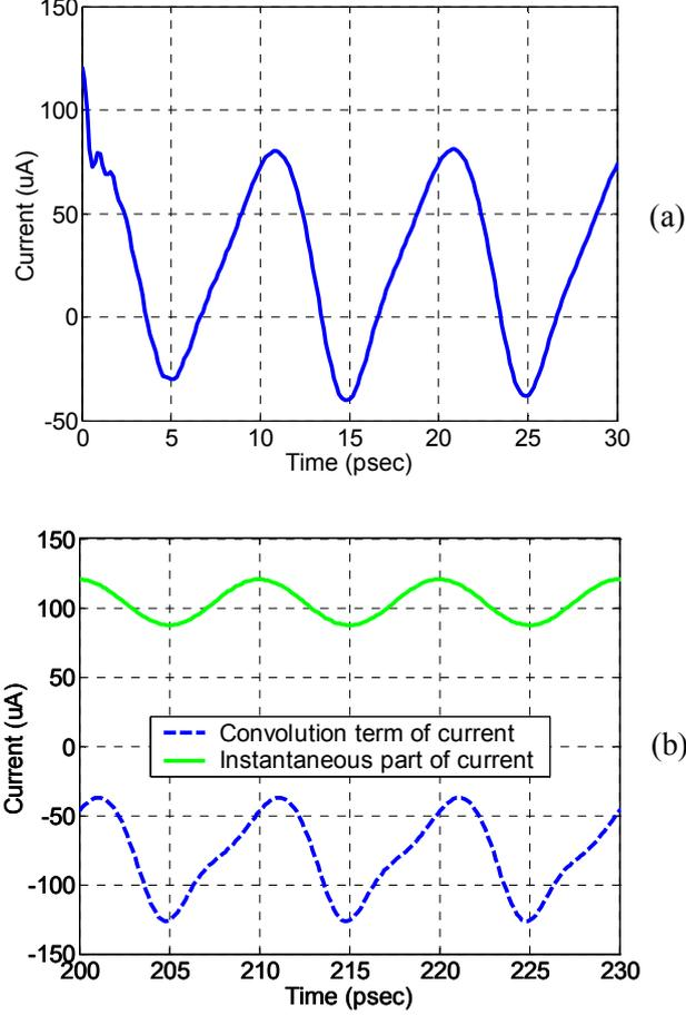
Fig. 4. (a) Transient response of the junction current when the DC bias voltage is centered on the first photon step and the LO is pumped at  $\alpha = 1$ . (b) Comparison of the two contributions of current once it has reached a steady state.
