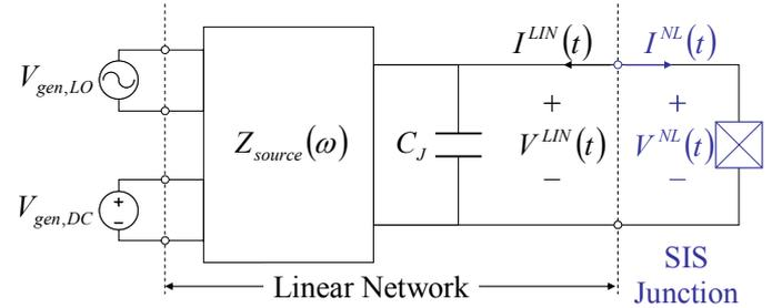
Fig. 5. Circuit describing the relation of the nonlinear diode current to the rest of the circuit in the voltage update algorithm [5]. The nonlinear current is transformed into the frequency domain and then linearly related to each harmonic of the LO.
