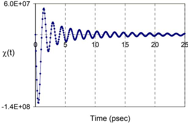
Fig. 2. The response function,  $\chi(t)$ , derived from the I-V curve data shown in Fig. 1b. The response function characterizes the nonlinearities and quantum-mechanical effects of the SIS junction in the time domain.
