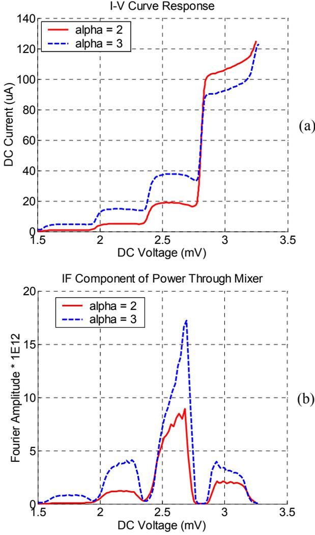
Fig. 8. (a) Pumped I-V curve response for two different source pumping strengths. The source impedance has been implemented as an ideal resistor of  $10 \Omega$ . (b) Two small signal tones, spaced at  $\pm 10$  GHz from the LO and with amplitude of  $hf_{LO} / 20e$ , were combined with the LO across the junction. The Fourier amplitude of the IF component of the power through the junction was extracted and plotted with respect to the DC voltage bias.
