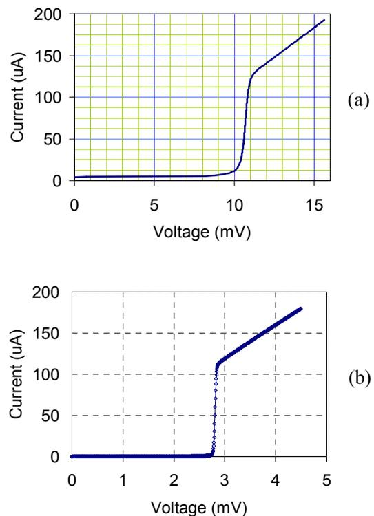
Fig. 1. Unpumped I-V curves that may be used for analysis. (a) Measured I-V curve for a series array of four Nb junctions. This is the typical response of the mixers used within the ALMA Band 3 receivers [7]. (b) I-V curve characteristic mimicking a measured response for a single Nb junction [9]. All MATLAB results contained herein are based on this fitted curve.
