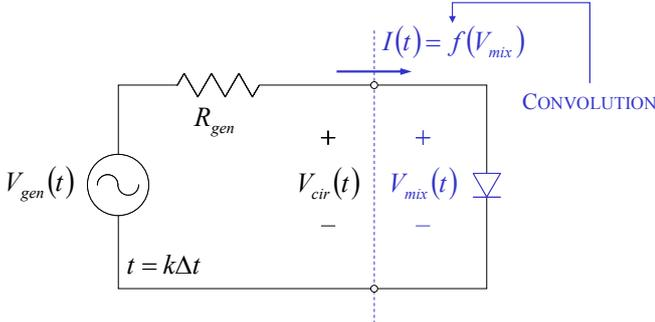
Fig. 6. Circuit describing the time domain voltage update method (TDVUM). The source impedance is represented here as a simple resistor, but may be a more complicated network. For each time step,  $\Delta t$ , the mixer voltage is iteratively matched to the circuit voltage at the terminal interface. However, since the quantum mixer current requires a convolution of previous voltage values, each iteration also requires a convolution. Note that  $V_{gen}$  includes the DC voltage bias.
