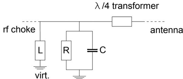
Fig. 5. Equivalent circuit of the tuning structure.
