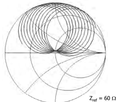
Fig. 3. Antenna impedances for frequencies between 200 and 260 GHz and a backshort distance of 30 mm. Smith chart is normalized to  $60 \Omega$ .
