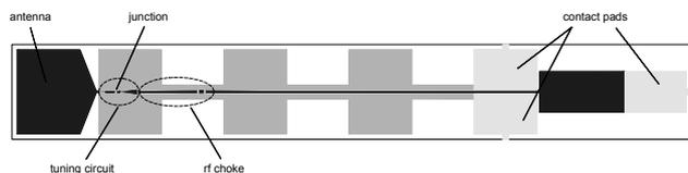
Fig. 1. Layout of the mixer chip with a size of  $2.5 \times 0.35 \times 0.1 \text{ mm}^3$ .
