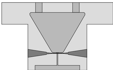
Fig. 3. One half of the mixer split block. The IF board pocket is in mid-grey and the back-to-back horns, waveguide and chip slot in dark-grey.
