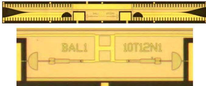
Fig. 4. Top, completed balanced finline mixer chip; Bottom, Enlarged image of circuits at the centre of the chip
