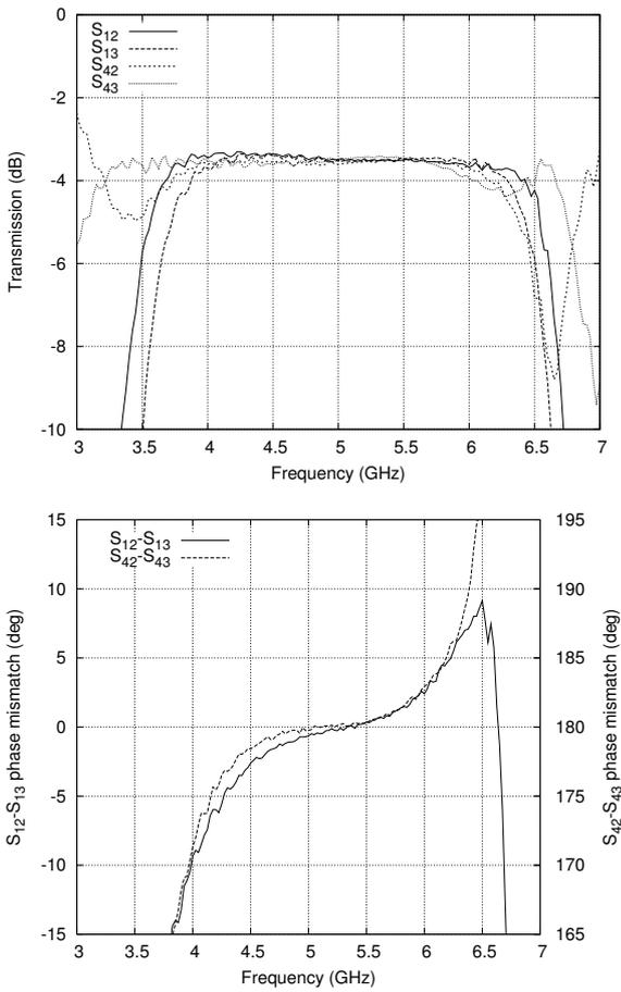
Fig. 10. Performance of the IF hybrid as measured at room temperature.
