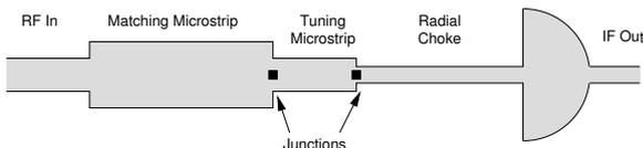
Fig. 8. Parallel junction tuning circuit.
