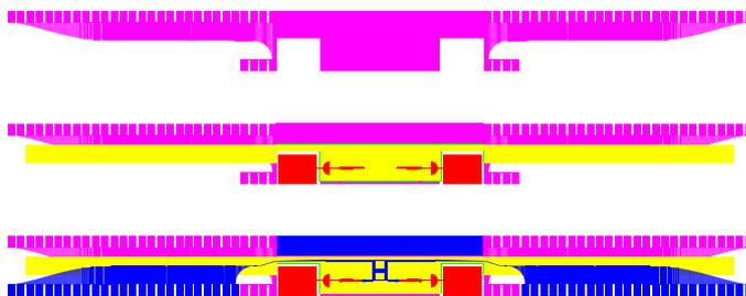
Fig. 5. Layers deposited during mixer chip fabrication. Top, ground-plane trilayer; Middle, ground-plane, insulation and junction definition layers and first wiring layer; Bottom, completed chip.
