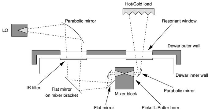
Fig. 11. Optical layout of the test receiver.
