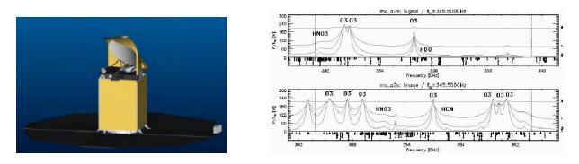
STEAM will measure molecular thermal emission spectra at sub-millimetre wavelengths. The instrument consists of a telescope that views thermal emission from the atmospheric limb imaged by a small linear array of receivers in the instrument platform. The incoming radiation from the Earth's limb is down converted in each mixer and amplified in low noise amplifiers. Spectrometers measure the spectral power density across each band.
