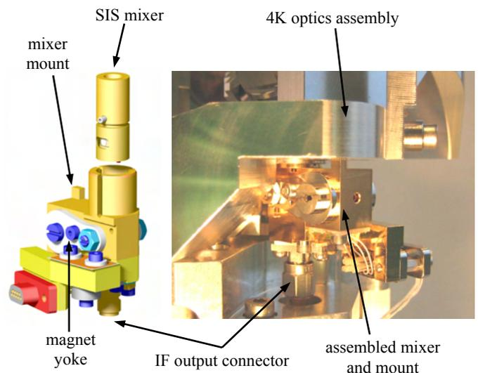
Fig. 5 – ALMA Band 9 mixer mount and mixer. (left) A 3-D model of the mixer and mixer mount. (right) An assembled mixer mounted in the 4K optics assembly of the first cartridge.
