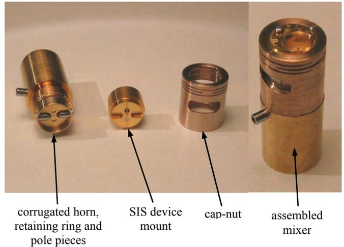
Fig. 4 – ALMA Band 9 SIS mixer. (left) The components of the mixer, including the new cap-nut with a multi-section spring cut into its walls. (right) The assembled mixer. The pin inserted into the horn is used for rotational alignment of the mixer in the mixer mount. (see Figure 5)
