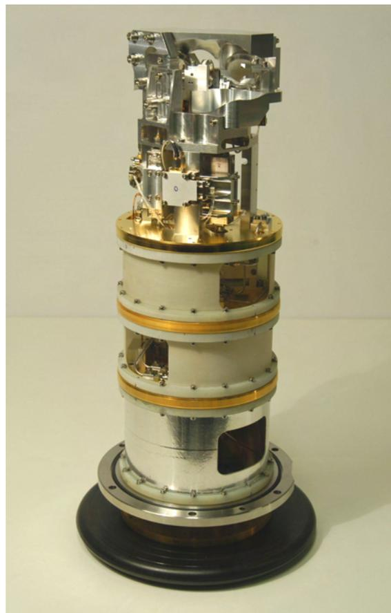
Fig. 7 – The first (prototype) ALMA Band 9 cartridge.
