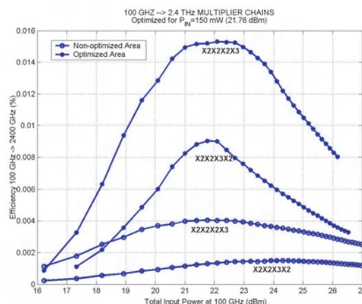
Fig. 1. Simulated and measured cascaded efficiency versus the power level at 100 GHz.
