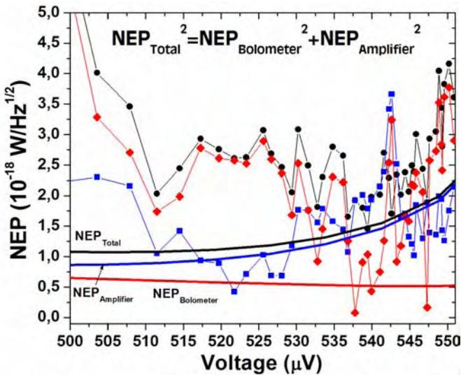
Fig. 7. The measured noise equivalent power ( $NEP$ ) near and below the superconducting gap voltage for  $f = 1.02$  kHz in comparison to theoretical prediction. In the region near the gap, there is a good qualitative agreement between experiment and theory.
