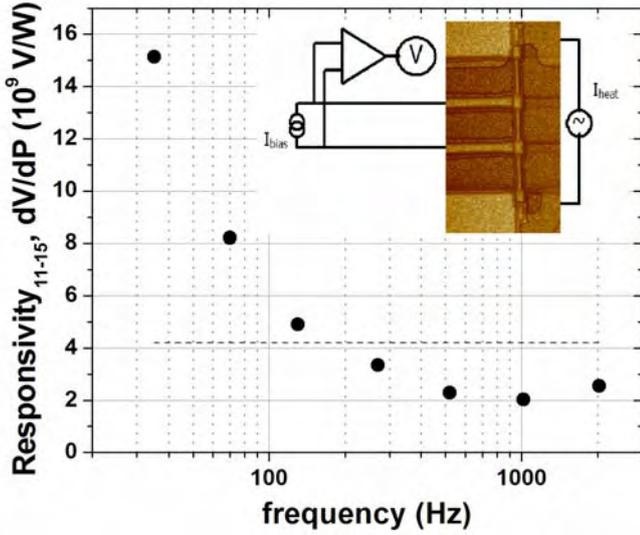
Fig. 4. Measured responsivity of the inner tunnel junctions at  $T_{ph}=100$  mK (circles) for modulation frequencies from 35 Hz to 2.02 kHz. Using the experimental parameters, the theoretical curve (dashed line) predicted a responsivity of  $4.2 \times 10^9$  V/W. (Inset) A view of the measurement scheme for responsivity.
