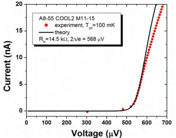
Fig. 3. Current-voltage characteristic of the tunnel junction used for response measurements (the inner pair) at  $T_{\text{ph}}=100 \text{ mK}$  (circles). The measured normal state resistance was  $14.5 \text{ k}\Omega$  and the subgap resistance was  $21.2 \text{ M}\Omega$ . The superconducting gap,  $2\Delta=568 \mu\text{eV}$ , was estimated by fitting the theoretical curve (solid line) with the experimental curve.
