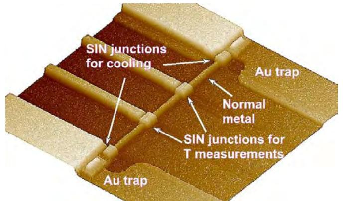
Fig. 2. Atomic force microscope image of a typical cold-electron bolometer. The outer SIN tunnel junctions cools the electrons in the normal metal. This electron cooling is enhanced by the Au traps in proximity to the cooling junctions. The inner SIN tunnel junctions acts as a thermometer to measure electron temperature in the absorber.
