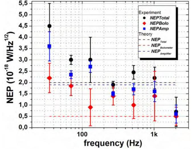
Fig. 6. Measured noise equivalent power ( $NEP$ ) of the inner tunnel junctions for modulation frequencies from 35 Hz to 2.02 kHz. The dashed lines show the theoretical estimations using the experimental parameters. The bolometer  $NEP$  is clearly better than  $10^{-19}$  W/Hz $^{1/2}$  for modulation frequencies above 100 Hz. Theory predicts  $5 \times 10^{-19}$  W/Hz $^{1/2}$  for the given experimental parameters.
