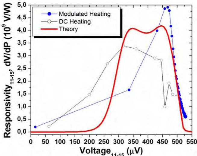
Fig. 5. Comparison between the two techniques of measuring the bolometer responsivity and the theoretical estimation. Very good agreement between experiment and theory can be seen in the region near and below the superconducting gap voltage.
