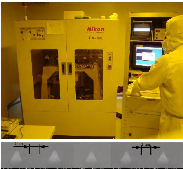
Fig. 2. The g-Line Stepper machine (top) and developed sub-micron photoresist patterns within one-shot exposing area of 3.5 \times 3.5 \text{ mm}^2 (bottom).
