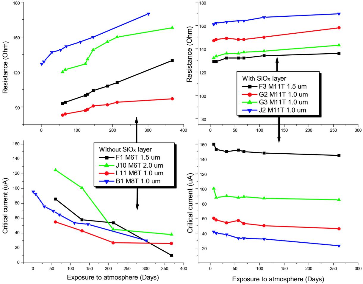
Fig. 5. Normal state resistance at 300 K (top panels) and critical current at 4.2 K (lower panels) versus exposure time in atmosphere at 300 K and 65 % RH. Left panels are for devices *without* passivation layer, right panels for devices *with* SiO<sub>x</sub> passivation layer.
