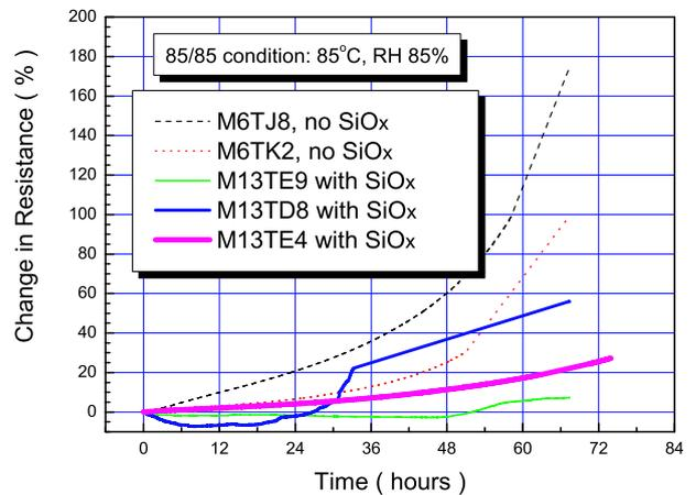
Fig. 7. Accelerated aging test by monitoring the device resistance under a harsh 85 °C - 85 % relative humidity environment as a function of time. The R<sub>300K</sub> of the devices is close to 150 Ω, except for device J8 which has a R<sub>300K</sub> of 100 Ω.
