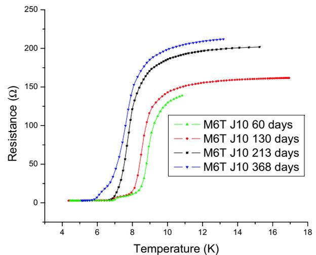
Fig. 3. Resistance versus Voltage plot of device J10 of batch M6T measured at several intervals, indicated in days after fabrication.
