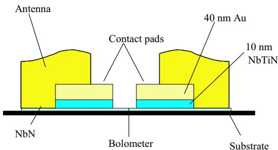
Fig. 2. Cross-sectional drawing of the HEB structure as shown from the top in Fig. 1. The cross-section reveals the composition of the contactpads, consisting of the NbN with  $10\text{ nm}$  NbTiN on top followed in situ by  $40\text{ nm}$  Au. Note that the resist protecting the NbN bridge is not shown.
