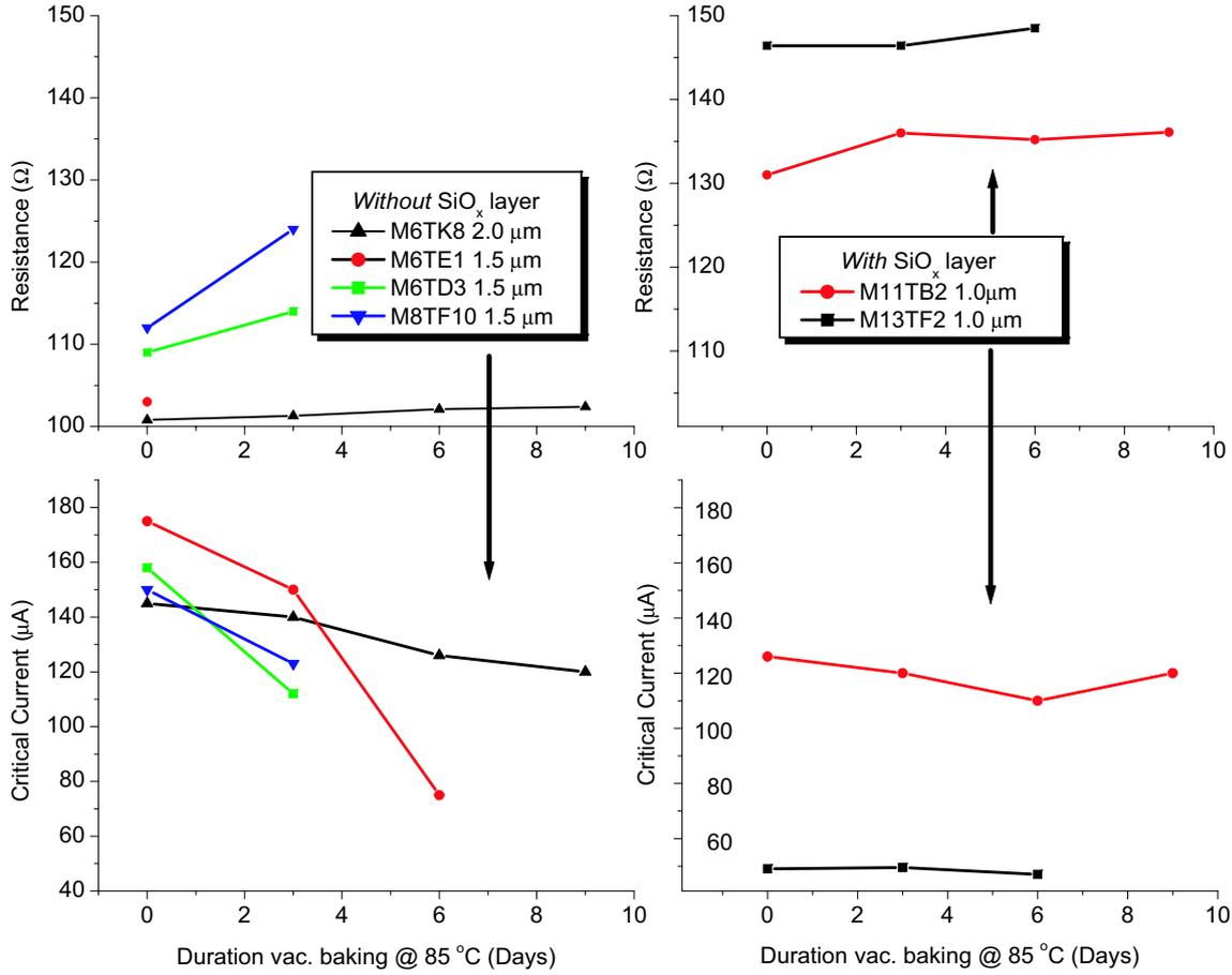
Fig. 6. Normal state resistance at 300 K (top panels) and critical current at 4.2 K (Lower panels) versus baking time in days at 85 °C and  $6 \cdot 10^{-5}$  mB. Left panels are for devices without passivation layer, right panels for devices with  $SiO_x$  passivation layer.
