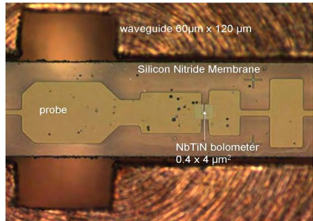
Fig. 3. 1.9 THz bolometer mixer with  $0.4 \times 4 \mu\text{m}$  NbTiN HEB device. The horn antenna is removed and the device metallization is seen through the backside of the transparent  $2 \mu\text{m}$  SiN membrane
