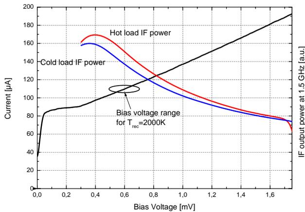
Fig. 6. Current-voltage (IV) curve of the 1.9 THz NbTiN waveguide HEB mixer with LO power at 1.75 THz. The HEB device size is  $0.4 \times 4 \mu\text{m}$ . Also shown is the IF output power in response to hot (295K) and cold (77K) loads placed at the receiver input.
