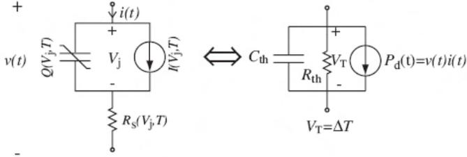
Fig. 2. Electrical equivalent (left) and electro-thermal equivalent circuit model (right) for harmonic balance simulations.
