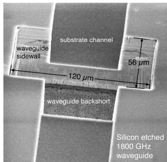
Fig. 4. SEM micrograph of a 1.9 THz two-level Si DRIE waveguide-substrate channel structure. Note that the dual masking process has been optimized to prevent formation of a burr between the waveguide and the substrate channel.
