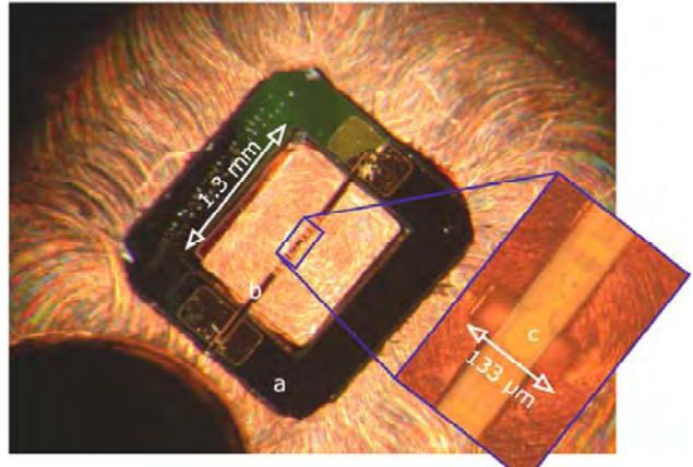
Fig. 1. Close-up of the center of a KOSMA 1.9 THz waveguide mixer block (feedhorn removed). Depicted are (a) the Si frame centering (b) the  $\text{Si}_3\text{N}_4$  membrane based superconducting HEB device in the substrate channel and (c) a close-up of the waveguide probe in the waveguide.
