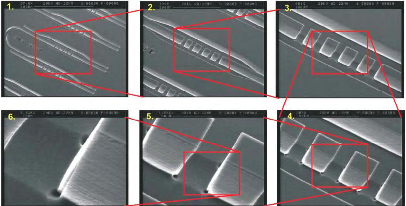
Fig. 3. SEM micrograph zoom in sequence onto a Si DRIE 1.9 THz branchline coupler. The scale bar on the last micrograph measures 10  $\mu\text{m}$ . Etch depth is 55  $\mu\text{m}$ . Note the low sidewall roughness of the Bosch process. The view is inclined by approx. 45°.
