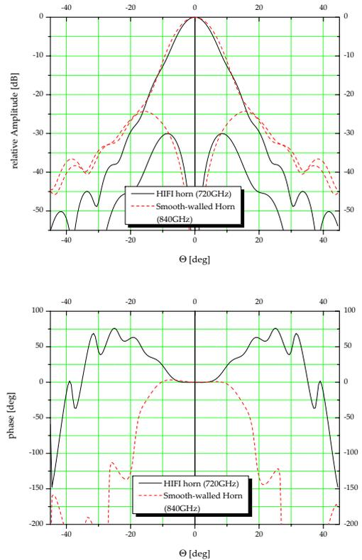
Fig. 7. The data of the smooth-walled horn compared to the data of the corrugated HIFI horn in D-plane. Both at their respective center frequency.
