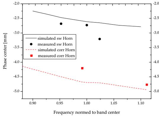
Fig. 8. Distance of phase center to horn aperture
