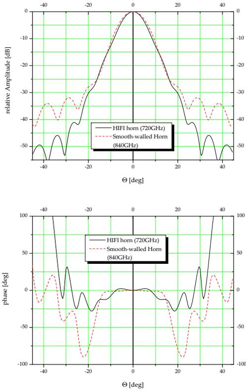
Fig. 5. The data of the smooth-walled horn compared to the data of the corrugated HIFI horn in E-plane. Both at their respective center frequency.
