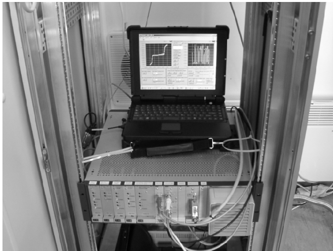
Fig. 12. View of the receiver control system, together with a test notebook.
