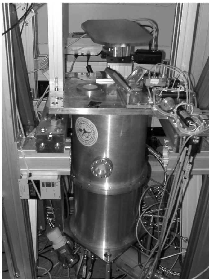
Fig. 2. View of the receiver after installation in the Apex telescope.
