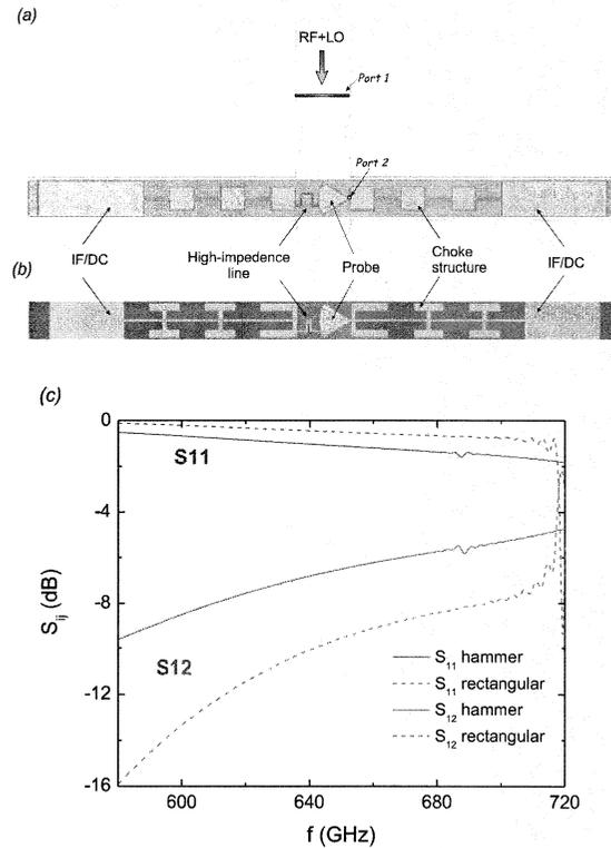
Fig. 4. (a) SIS design with a rectangular choke structure. The figure also shows the cavity where the junction will be placed. (b) SIS design with a hammer type choke. (c) Results of the simulations for the two types of choke structures.
