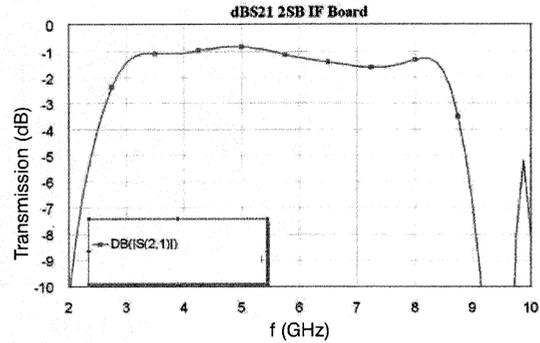
Fig. 3. Simulated transmission of the IF circuit.
