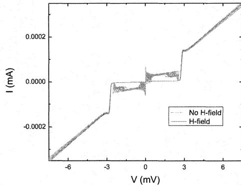
Fig. 5. IV curves of 12 different junctions intended to be used in the 2SB mixer. Notice the good repeatability necessary for a good performance of the mixer.
