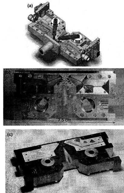
Fig. 1. (a) Proposed design of a 2SB mixer for ALMA band 9. (b) Micromachining realization of the mixer. (c) Mixer with the IF circuit board and magnets.
