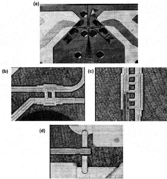
Fig. 2. (a) Detailed view of the RF components of the mixer. (b) LO injector. (c) RF quadrature hybrid. (d) Room for the mixers.
