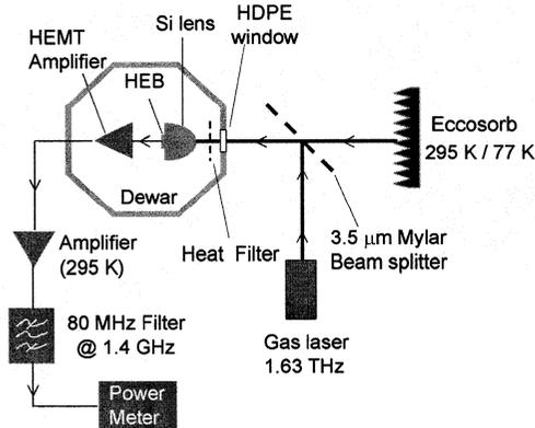
FIG 4. Heterodyne test setup used for the measurements in figure 5.
