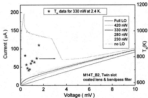
FIG 6. Current-voltage characteristics (full lines, left axis) of the twin slot antenna coupled NbN HEB mixer without and with radiation from the QCL at 1.6 THz. The receiver noise temperature  $T_{rec}$  (symbols, right axis) versus the bias voltage for the optimal LO power at the HEB, which was measured at a reduced bath temperature of 2.4 K and with an additional bandpass filter centred at 1.6 THz.
