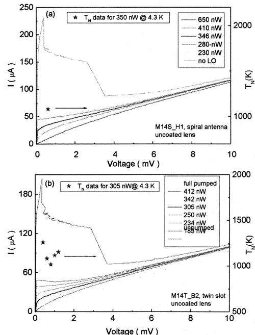
FIG.5. Current-voltage characteristics (full lines, left axis) of a NbN HEB mixer without and with radiation from the QCL at 1.6 THz. The measured receiver noise temperature  $T_{\text{rec}}$  (symbols, right axis) versus the bias voltage for the optimal LO power at the HEB. (a) for the spiral antenna mixer, while (b) for the twin-slot mixer.
