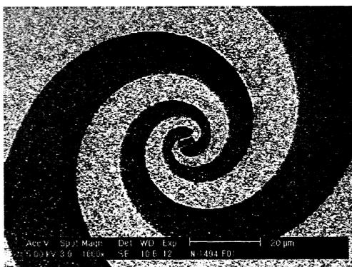
FIG. 1 SEM micrograph of a self-complementary spiral antenna coupled HEB mixer on Si substrate. The NbN HEB has a width of 2  $\mu\text{m}$  and a length of 0.2  $\mu\text{m}$ , giving a low temperature normal state resistance of 96  $\Omega$ . The dark part in the center is a remaining e-beam resist, which is used to define the width of the HEB.
