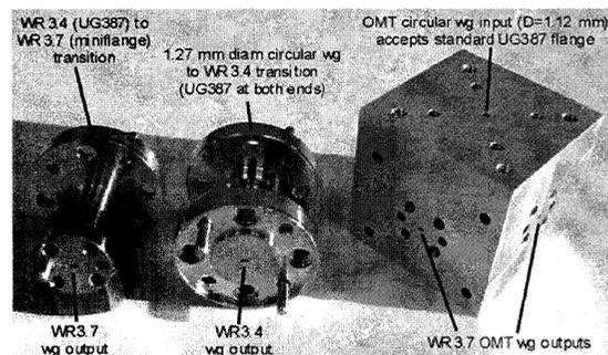
Fig. 2. View of assembled OMT (on the right) with the circular waveguide input on top and the two WR3.7 waveguide outputs with custom mini-flanges. Two of the 19.05 mm long transitions used for testing are shown to the left of the OMT.
