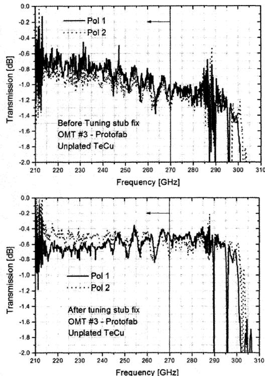
Fig. 8. Pol 1 and Pol 2 transmission measurement of OMT n. 3 before (top) and after (bottom) tuning stub fix. The vertical line in the graphs delimits the nominal highest frequency of the band at 270 GHz.
