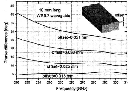
Fig. 11. Transmission phase differences between a straight 10 mm long WR3.7 waveguide and a same length waveguide section where block halves are offset by 0.013 mm, 0.025 mm, 0.038 mm, 0.051 mm.
