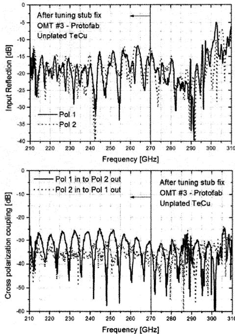
Fig. 9. Pol 1 and Pol 2 input reflection (top), and cross polarization coupling (bottom) of OMT n. 3 after tuning stub fix.
