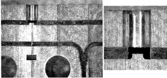
Fig. 4. OMT n. 5 machined at Univ. of Arizona. View of an assembled mating pair of blocks showing the internal waveguide circuitry of turnstile junction, and power combiner (on the left), and the details of the tuning stub at the turnstile junction circular waveguide base (on the right).
