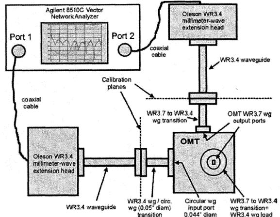
Fig. 5. S-parameter measurement of the OMT with the VNA. The particular configuration refers to the cross-polarization measurement.
