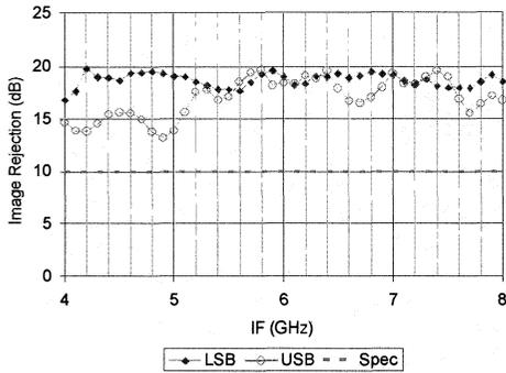
Fig 4: Image Rejection of the Pol 0, LSB and USB, in narrow band mode, at LO=100 GHz.
