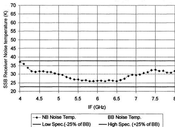
Fig 3: Narrow band noise temperature at LO=100 GHz, Mixer at 4.00K, Pol 0-USB
