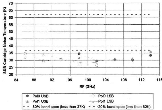
Fig 2. Band 3 Receiver broadband noise temperature
