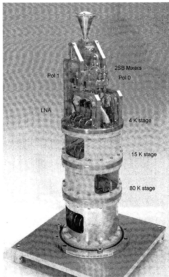
Fig. 1: Photograph of the Band 3 cartridge (height is 508.5 mm)
