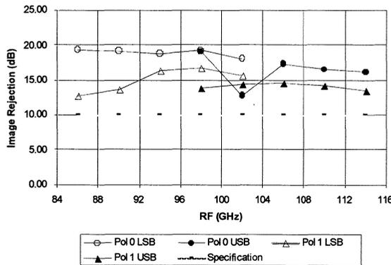
Fig. 5: Image rejection of the four channels
