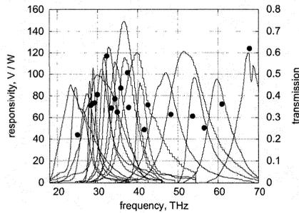
Fig. 5. The dependence of the receiver's responsivity versus frequency (filled circles) and the transmissions of the bandpass filters used in the experiment (lines).
