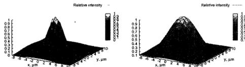
Fig. 3. Simulated intensity of LO spot on the NbN sensitive bridge at 30 THz. The left graph corresponds to the flat wave front, while the right graph corresponds to the situation when the LO spot is slightly defocused. The dimensions of  $x$ - $y$  planes shown in the images are close to the in-plane dimensions of NbN sensitive bridge. The simulation are given for hemispherical Ge lens with the diameter of 12 mm and extension length of 1.96 mm.
