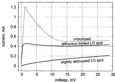
Fig. 4. IV – curves versus LO spot for directly coupled NbN HEB.
