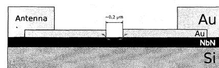
Fig. 1. RF current in the contacts between sensitive NbN bridge and Au antenna. The small area where RF current flows is denoted by the arrows.
