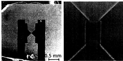
Fig. 2. SEM photos of directly lens coupled NbN HEB mixer.
