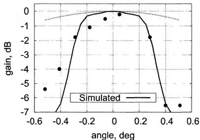
Fig. 6. Radiation pattern of directly coupled NbN HEB mixer based receiver at 30 THz (solid circles). Dotted line corresponds to the radiation pattern of the system consisting of Si lens, spiral antenna and a mixer at 2.5 THz [8]. Solid line corresponds to the simulation given for hemispherical Ge lens with the diameter of 12 mm and extension length of 1.96 mm. More detailed description of the receiver is given in [6].
