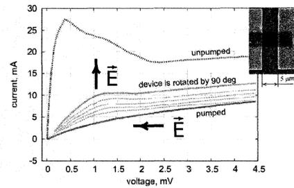
Fig. 7. LO pumped IV-curves for  $5 \times 5 \mu\text{m}^2$  device at 10.7 THz.
