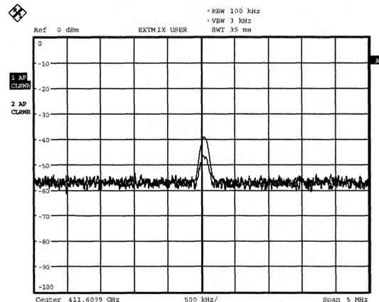
Fig. 7. Spectrum of a free-running InP Gunn device oscillator in a third-harmonic mode. RF power level: 0.04 mW, center frequency: 411.610 GHz, vertical scale: 10 dB/div, horizontal scale: 500 kHz/div, resolution bandwidth: 100 kHz, video bandwidth: 3 kHz, reference level not calibrated.
