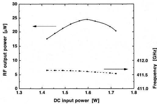
Fig. 8. Uncorrected RF power level readings of an InP Gunn device in a third-harmonic mode at 411.6 GHz as a function of the applied bias.  $\bullet$ : RF output power in a third-harmonic mode;  $\blacksquare$ : third-harmonic oscillation frequency.
