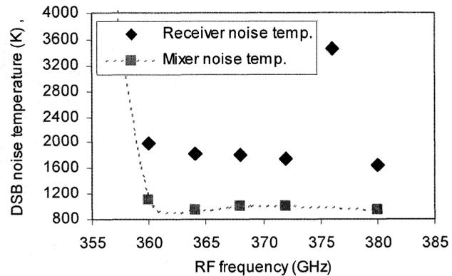
Fig.5. Measured DSB receiver and mixer noise temperature VS frequency. Degradation in the receiver noise temperature noticeable at 376 GHz is due to a sharp resonance in the LO signal coupling between the doubler and the mixer. Inserting an isolator between the mixer and the doubler would cancel the resonance.
