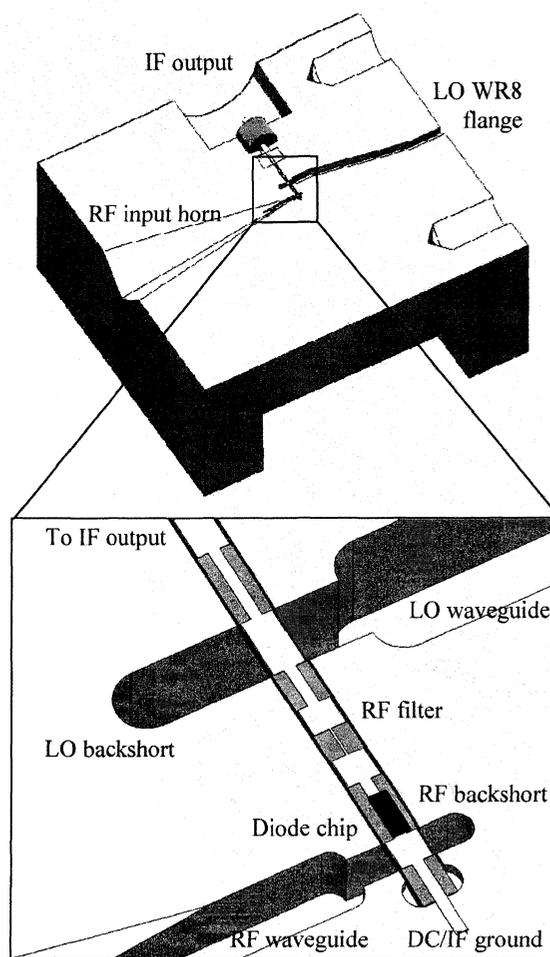
Fig. 1. Schematic view of the 380 GHz SHP mixer circuit mounted into the lower half of the mechanical waveguide split block. The circuit has been optimized for best performances with an anti-parallel pair of planar Schottky diodes from VDI.
