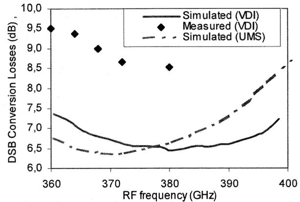
Fig.3. Predicted DSB conversion losses of the 380 GHz SHP mixer designed to incorporate an anti-parallel pair of Schottky diodes from VDI (full curve), along with the predicted performances of a similar mixer circuit incorporating UMS-type anti-parallel pair of planar Schottky diodes (dashed curve). Measured mixer conversion losses using a VDI diodes pair are shown (dots) for comparison.
