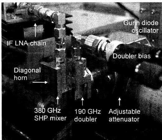
Fig.4b. View of the test setup showing the 190 GHz fixed-tuned doubler connected to the 380 GHz fixed-tuned SHP mixer. A waveguide attenuator is inserted between the doubler and the Gunn oscillator. The IF signal from the SHP mixer is output to a LNA IF chain.
