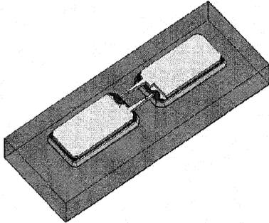
Fig.2a. Schematic view of the planar Schottky diodes from VDI (Ref. SC1T9-D20). The chip includes two air-bridges. Electrical parameters are:  $R_s=10 \Omega$ ,  $\eta=1.25$ ,  $C_{j0}=2.5 \text{ fF}$ ,  $I_{\text{sat}}=30 \text{ fA}$ ,  $V_{\text{bi}}=0.8 \text{ V}$ ,  $A=1.76 \mu\text{m}^2$ .
