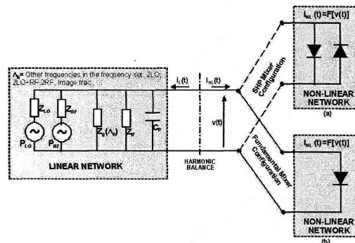
Fig. 1. Block diagram of the analyzed circuit for a SHP antiparallel diode pair (a) and a fundamental Schottky mixer (b).
