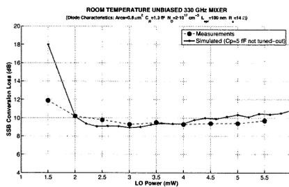
Fig. 10. Comparison between measurements and simulations for a 330 GHz SHP antiparallel-diode pair Schottky mixer [7].
