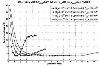
Fig. 3. Influence of epilayer doping in the SSB conversion loss of the 400 GHz fundamental mixer at room temperature. No parasitics have been considered ( $C_p=0$  fF).
