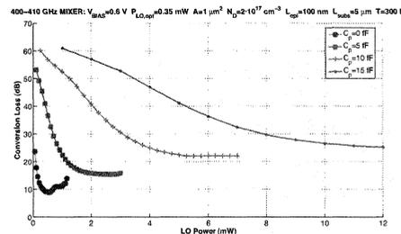
Fig. 5. Influence of the parasitic capacitance in the SSB conversion loss of the 400 GHz fundamental mixer at room temperature. IF optimized at  $C_p=0$  fF and  $P_{LO}=0.35$  mW.
