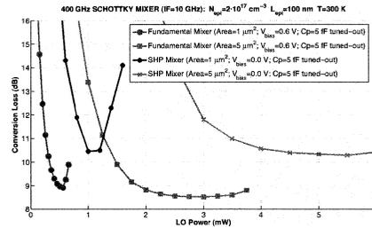
Fig. 8. Comparison between the performances of the 400 GHz fundamental Schottky mixer and the 400 GHz SHP antiparallel-pair Schottky diode mixer.
