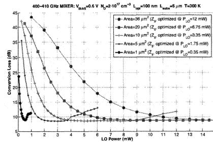
Fig. 4. Influence of anode area in the SSB conversion loss of the 400 GHz fundamental mixer at room temperature. No parasitics have been considered ( $C_p=0$  fF).
