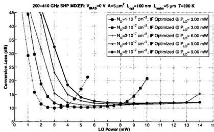
Fig. 6. Influence of epilayer doping in the SSB conversion loss of the 400 GHz SHP mixer at room temperature. No parasitics have been considered ( $C_p=0$  fF)
