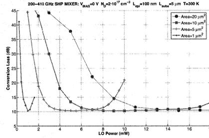
Fig. 7. Influence of anode area in the SSB conversion loss of the 400 GHz SHP mixer at room temperature. No parasitics have been considered ( $C_p=0$  fF)
