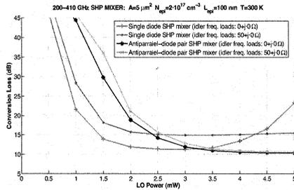
Fig. 9. Comparison between the performances of the 400 GHz fundamental Schottky mixer and the 400 GHz SHP antiparallel-pair Schottky diode mixer. Influence of the impedances at idler frequencies.
