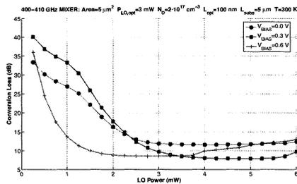
Fig. 2. Influence of bias in the single-side band (SSB) conversion loss of the 400 GHz fundamental mixer at room temperature. No parasitics have been considered ( $C_p=0$  fF). IF optimized at 3 mW LO power.
