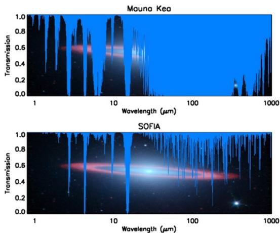
**Figure 1. The comparison of atmospheric transmission at THz frequencies between ground based and airborne facilities. Note that THz observations (1 – 10 THz) are completely blocked by the effects of atmospheric water vapor.**
