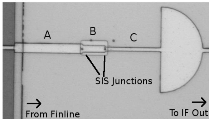
Fig. 3. The dual junction tuned mixer and radial RF-choke design. Typical dimensions are: A 7 x 48.5 μm, B 5 x 15.5 μm and C 3 x 39 μm.
