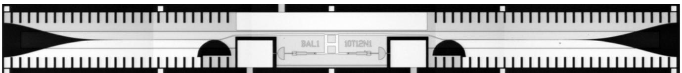
Fig. 17. A 700 GHz single chip balanced SIS mixer, based on back-to-back finline tapers. The RF and LO signals are fed via the two finline tapers and combined in microstrip quadrature hybrid at the center of the chip.
