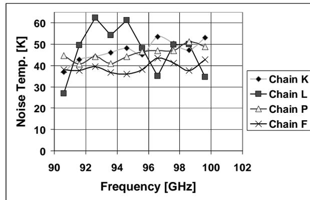
Figure 5: Measured noise temperature of four LNA chains.
