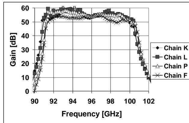
Figure 4: Measured gain of four LNA chains.
