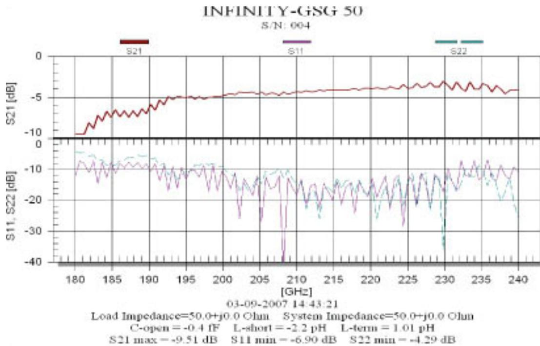
WR-03 Wafer Probe S/N004 on WR-05 System
