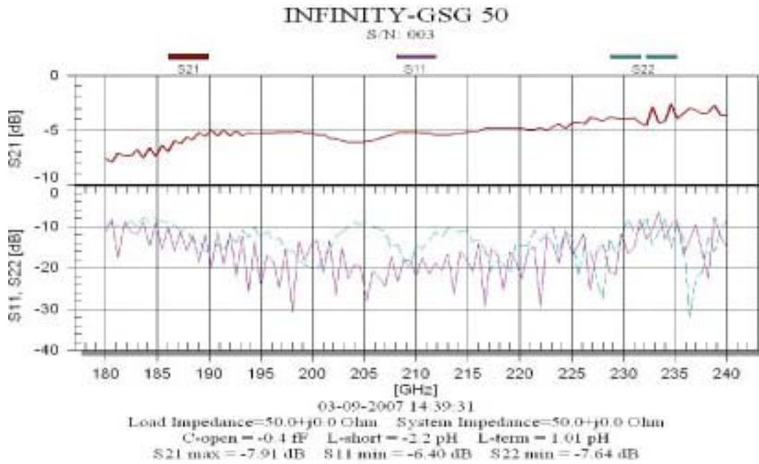
WR-03 Wafer Probe S/N003 on WR-05 System
