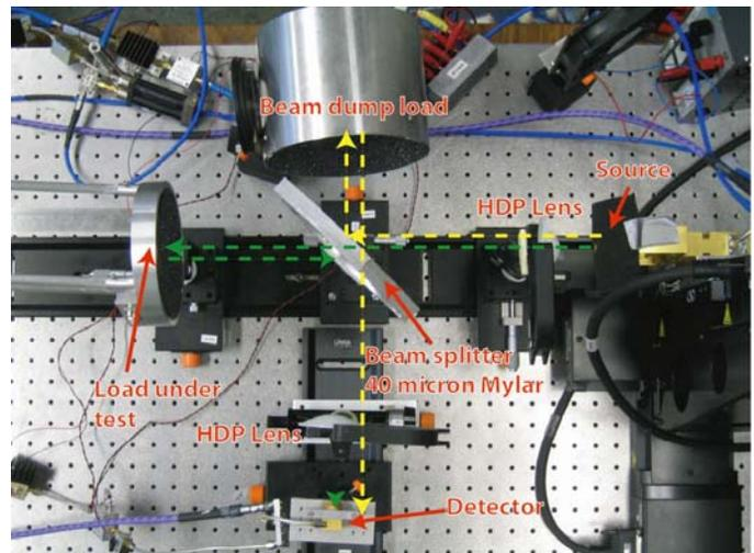
Fig. 1. Layout of single port quasi-optical VNA
