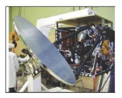
and increased reliability. Both bands share pre-optics and calibration targets. We expect the PREMIER radio telescope to be similar to the Odin telescope which is a shaped off axis Gregorian design. It will be constructed of carbon fibre composite material for thermal stability and have a surface accuracy better than 15 µm RMS, a factor of 2 less demanding than for Odin.
