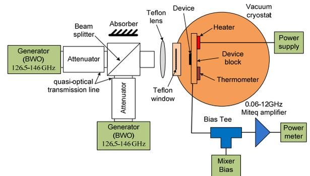
Fig. 2 The intermediate frequency gain bandwidth measurement setup
