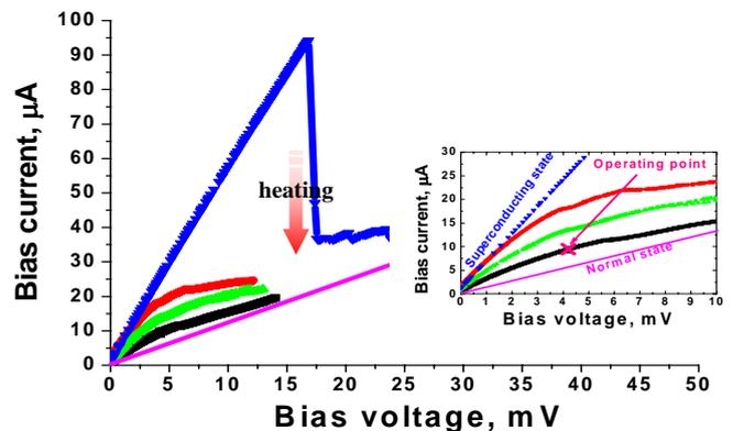
Fig. 3 Set of dc voltage bias characteristics (increasing from top to bottom) levels of the LO power. The upper curve was taken without LO power.
