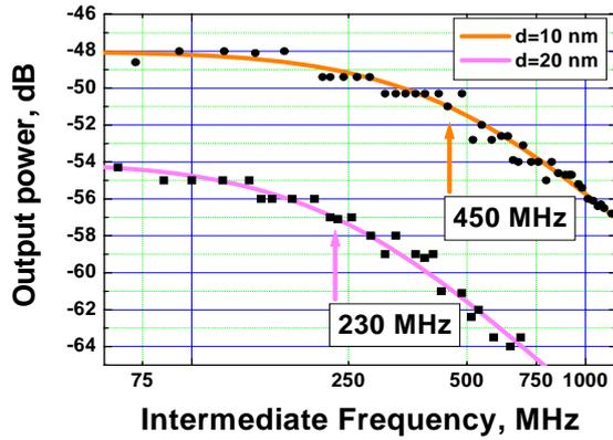
Fig. 4 The output signal vs IF bandwidth for NbZr bridges 10nm and 20nm thick. The 3 dB roll-off frequency is marketed for all curves. The fitting lines are obtained from (1).
