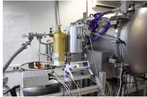
Fig. 2. At the left a cryostat with a vacuum Hot/Cold load is shown, which is coupled via a gas cell and the large reimager vacuum tank to the FPU cryostat.
