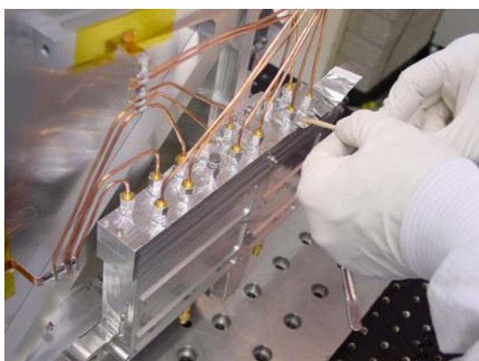
Fig. 6. The IF amplifier housing being covered with Al tape. An additional box was produced that facilitated the wrapping of the IF connectors.
