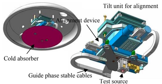
Fig. 7 Drawings of the beam scanning system
