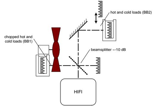
Fig. 9 Measurement setup for the linearity experiments
