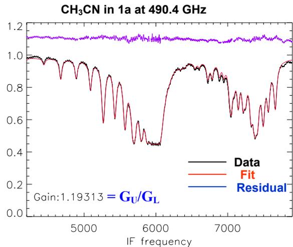
Fig. 19 Example of side-band ratio retrieval based on modelled line profile fitting on a transition of CH<sub>3</sub>CN in band 1a.
