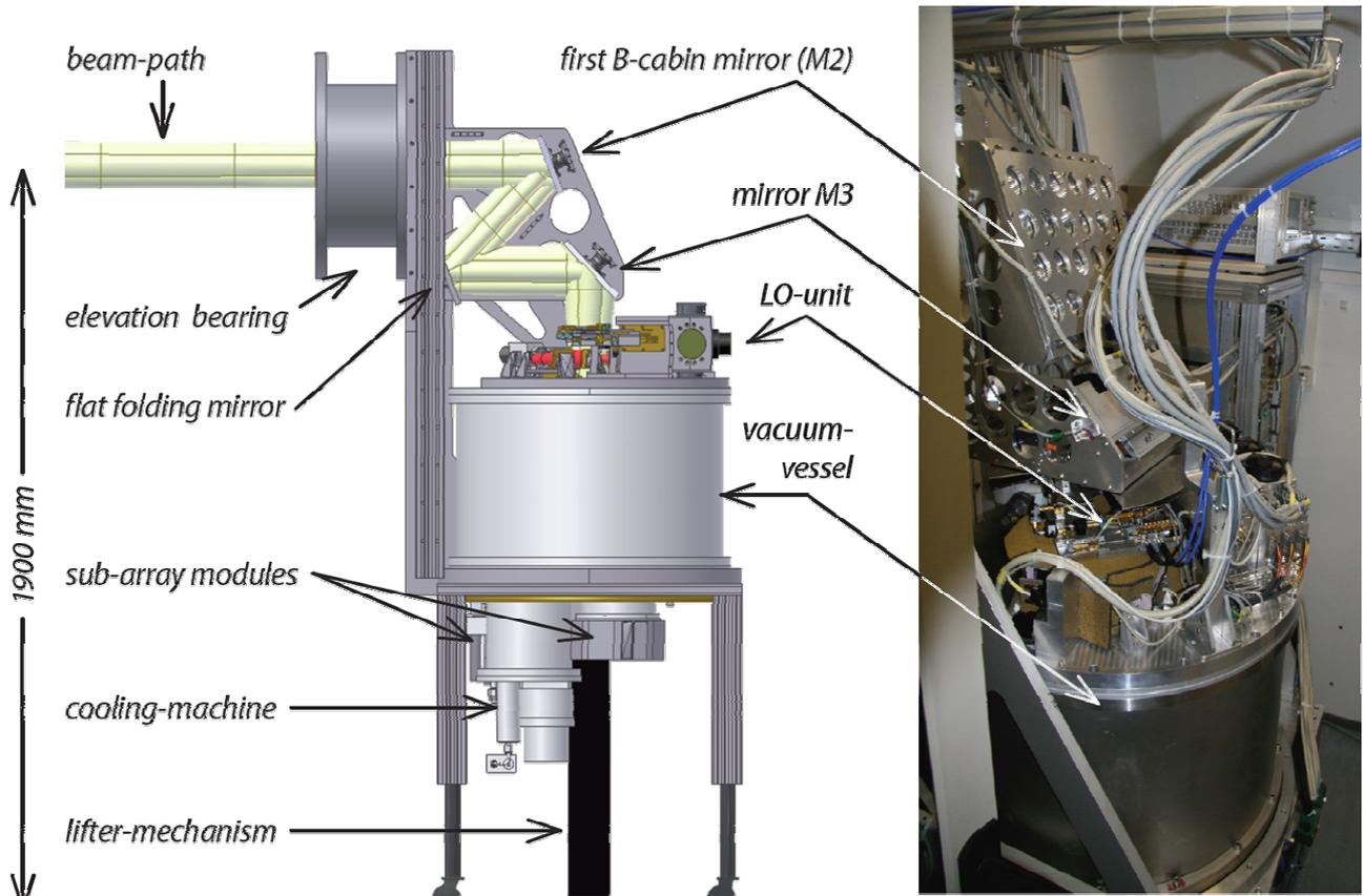
Fig. 2: System overview (CAD 3D model – left hand side) and photograph of CHAMP<sup>++</sup> as mounted in the Nasmyth B-cabin of the telescope.
