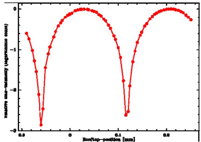
Fig. 7: Relative line intensity of a harmonic mixer RF-signal, injected into the receiver signal path, versus SSB roof-top position.
