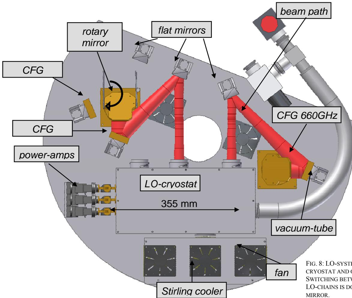
FIG. 8: LO-SYSTEM WITH LO-CRYOSTAT AND OPTICS PATH (RED). SWITCHING BETWEEN THE TWO HFA LO-CHAINS IS DONE BY A ROTARY MIRROR.
