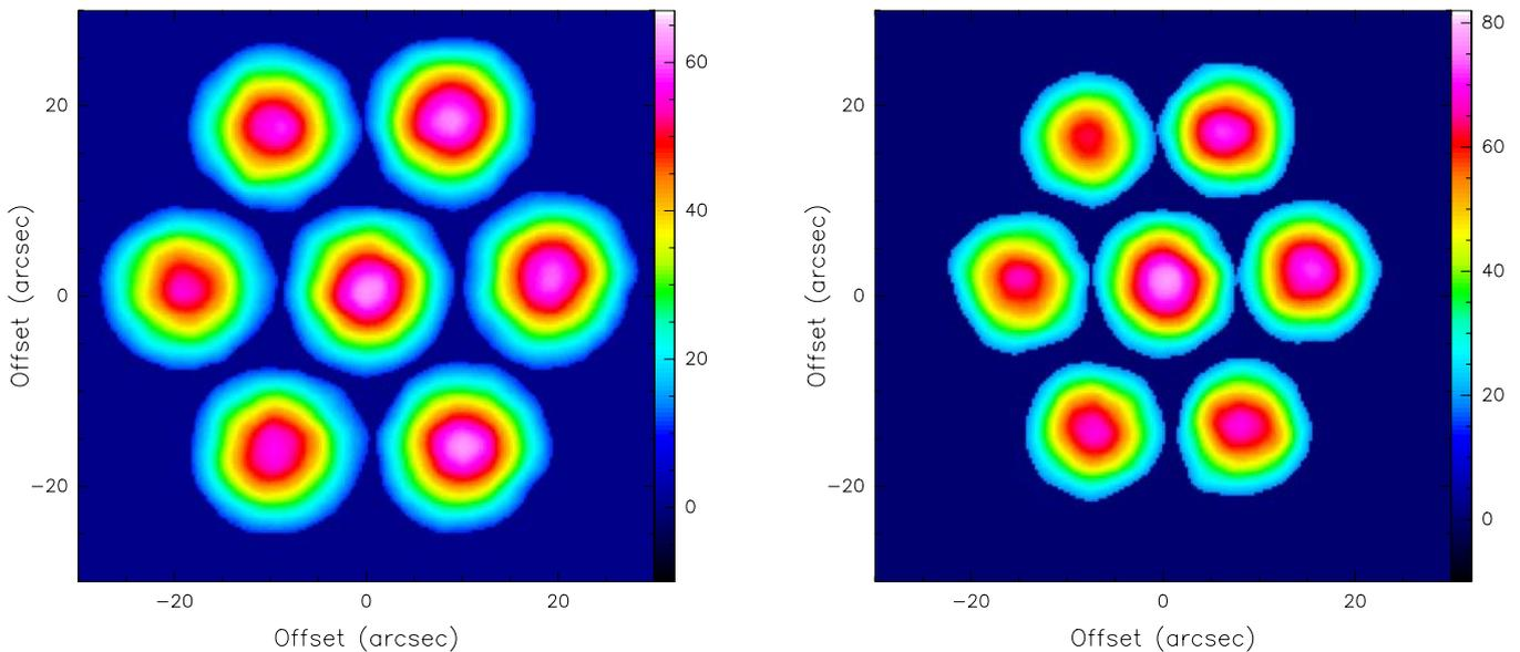
FIG. 11: CHAMP<sup>+</sup> BEAM PATTERN AS OBTAINED TOWARDS MARS (IN TOTAL POWER SCANNING MODE). LEFT HAND SIDE: LFA; RIGHT HAND SIDE: HFA. POSITIONS AND SHAPE AGREE WELL WITH DESIGN-VALUES, WHILE THE ARRAY IS NEARLY INVARIANT AGAINST ROTATION OF THE 60° SYMMETRY ANGLE.
