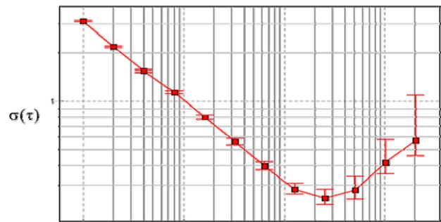
FIG. 10: TYPICAL ALLAN-PLOT HERE FROM ONE OF THE HFA CHANNELS SHOWING APPROX. 200S ALLAN MINIMUM TIME AT A SPECTROSCOPIC RESOLUTION OF 1MHZ.
