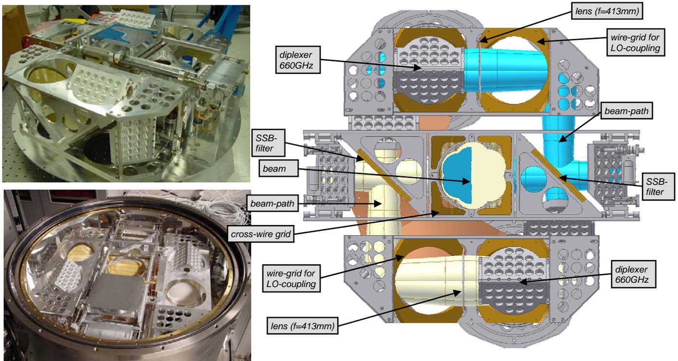
Fig. 4: Cold-optics assembly, including the filter elements (SSB-filter and LO-diplexer), wire-grids and lenses.
