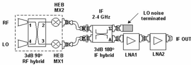
Fig. 1. Layout of the waveguide balanced HEB mixer.
