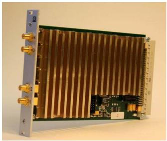
Omnisys has an FFT spectrometer design optimized for ground based applications. It follows the single Eurocard standard size and provides up to 2 GHz bandwidth and 1-4 inputs. With four inputs, the maximum processed bandwidth is 500 MHz.
