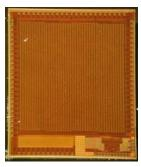
HIFAS, Omnisys fifth generation autocorrelation spectrometer ASIC is being developed. It is a full-custom design with over two million transistors, designed for IBM's 180 nm SiGe Bi-CMOS process. Unlike earlier generations, it contains both the bipolar 3-level ("1.5-bit") A/D converter and the CMOS correlator on the same chip. Thereby, the sensitive high-speed digital interface between the two parts gets integrated on the chip.
