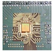
The goal is to reach a bandwidth of 8 GHz, a resolution of 1024 channels, and a power consumption of 3-4 W. When finished, this chip will set a new world record in autocorrelator performance, and open for new possibilities in radiometry on both space and ground.
