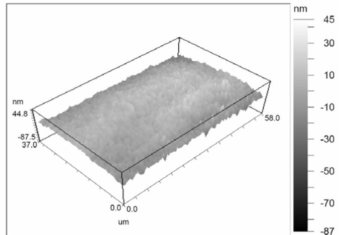
Fig. 2. Surface roughness measurement at the bottom of the back-short structure. The roughness scale is at the right.
