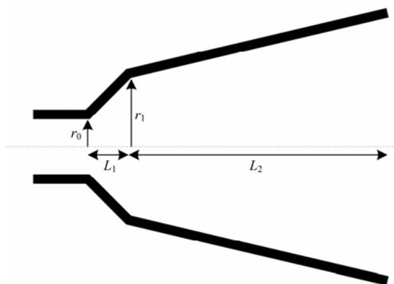
Fig. 1. Geometry of the dual-mode two-section horn with a flare angle discontinuity.  $r_0$  is the radius of the circular waveguide.  $r_1$  and  $L_1$  are the radius and the length of the first conical section.  $L_2$  is the length of the second conical section.
