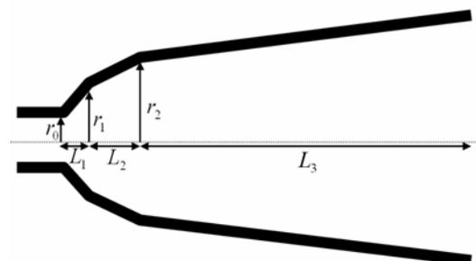
Fig. 2 Cross section of a three-section horn. r<sub>0</sub> is the radius of the circular waveguide. r<sub>1</sub> and L<sub>1</sub> are the radius and the length of the first conical
