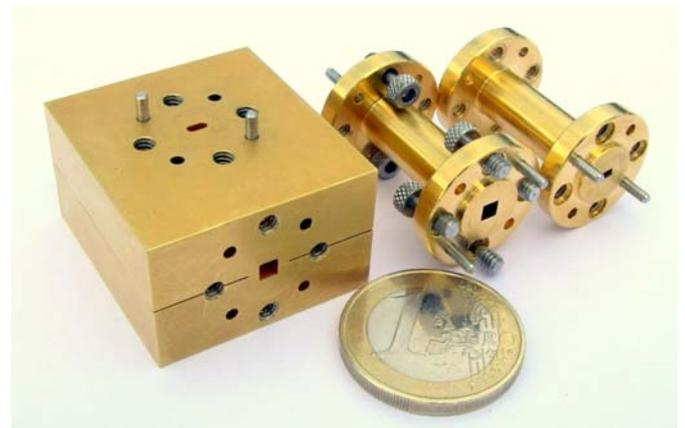
Fig. 12. Photograph of the assembled OMT (left) showing the square waveguide input and the oval waveguide output. The external dimensions are  $19 \times 30 \times 33 \text{ mm}^3$ . Standard UG387 flanges are used at all ports. The two identical square-to-WR10 waveguide transitions used to test the OMT are shown on the right.
