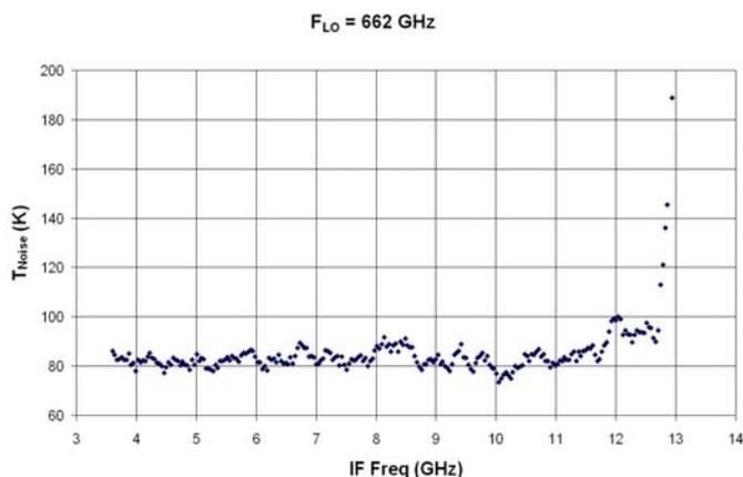
Fig. 2 IF coverage for the AlN mixer using an LO frequency of 662 GHz. For obtaining data over the whole 600 - 720 GHz range, the LO frequency
