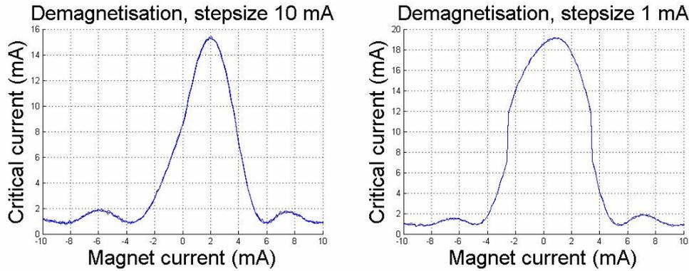
Figure 6: Demagnetization with a step size of 10 mA (common for ALMA  $\text{AlO}_x$  mixers) results in a asymmetric curve (left hand side). Demagnetization with a step size of 1 mA results in an almost symmetric curve (right hand side). Both curves were obtained using an  $\text{AlO}_x$  barrier and a starting amplitude of 40 mA. Demagnetizing was always followed by defluxing.
