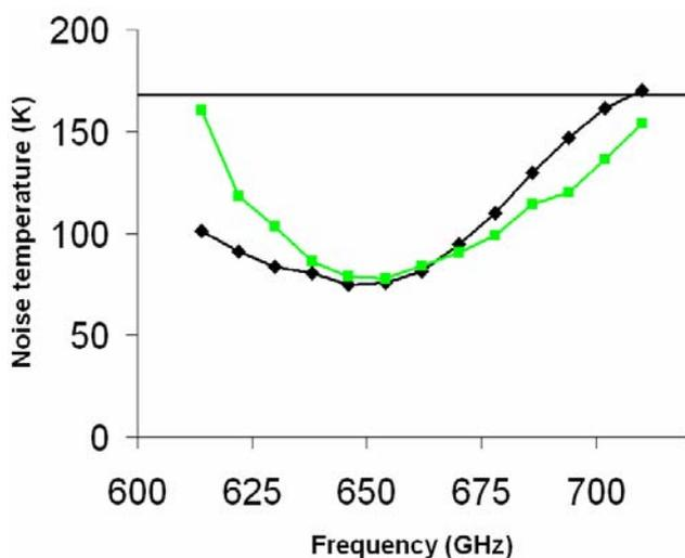
Fig. 9 Noise temperatures of present mixers based on AlO<sub>x</sub> (green line) and AlN (black line) barriers. The AlO<sub>x</sub> barrier mixer is one of the delivered junctions for ALMA. It has a size of 1 μm<sup>2</sup> and a resistance times area of 25 Ω μm<sup>2</sup>. The AlN barrier mixer has a size of 0.25 μm<sup>2</sup> and a resistance times area of 3.7 Ω μm<sup>2</sup>. The AlN mixer has a lower minimum noise temperature.
