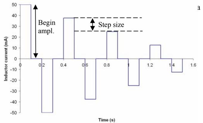
Fig. 5 Block shaped current function with decreasing amplitude used for demagnetizing the magnet. The step size is the amplitude decrease between two succeeding current pulses of the same sign. Each negative current pulse has the same amplitude as the previous positive pulse.
