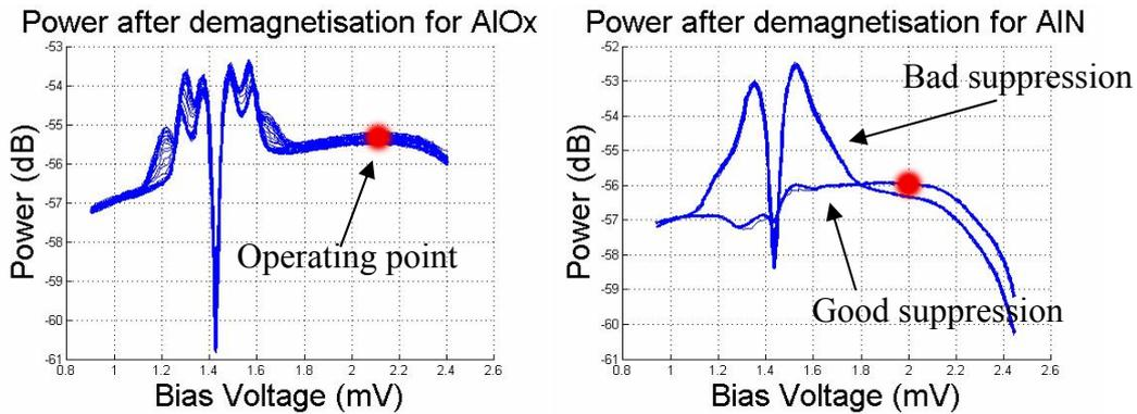
Figure 7: Measured power v.s. bias voltage profile after demagnetization and defluxing for an  $\text{AlO}_x$  and the  $\text{AlN}$  mixer. The operation procedure was repeated 40 times for each mixer. For  $\text{AlO}_x$  all attempts did result in a good operating point (the red dot). For  $\text{AlN}$  in 21 cases the Josephson effect was insufficiently suppressed. The starting amplitude of demagnetization was 40 mA and the step size was 1 mA.
