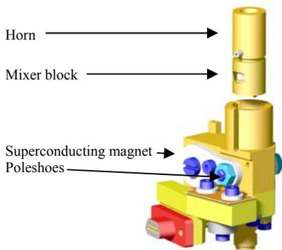
Fig. 4 Mixer holder with superconducting magnet, poleshoes, heater contact, thermometer and IF connector. To operate an AlN barrier mixer the remanent field inside the magnet and the flux inside the superconducting material should be removed. After this, the right magnetic field can be set to suppress the Josephson effect (Figure by Gerrit Gerlofsma).
