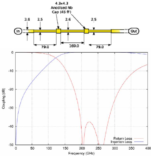
Fig. 14. (Top) Diagram of the RF band-pass filter. Dimensions are in microns. (Bottom) Calculated scattering parameters of the RF band-pass filter.
