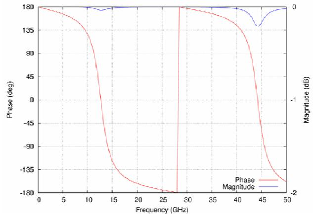
Fig. 13. Phase and magnitude of the reflection back from the finline taper towards the SIS junction in the IF band, as calculated by HFSS.
