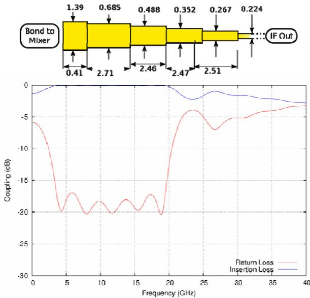
Fig. 19. (Top) Diagram of the IF output transformer, fabricated on 0.254 mm thick Duroid 6010LM. Dimensions are in mm. (Bottom) Combined scattering parameters of the IF connection and output transformer, normalised to 16.5  $\Omega$  at the input and 50  $\Omega$  at the output.
