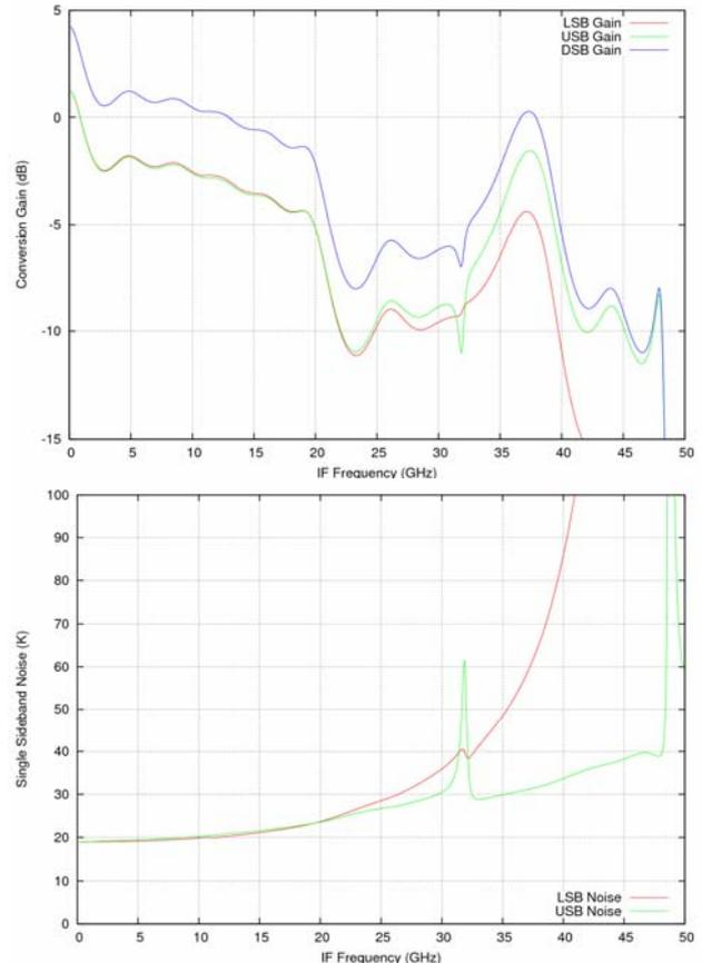
Fig. 22. SuperMix calculated mixer conversion gain (top) and noise temperature (bottom) against IF frequency for the complete single-junction mixer. The mixer is biased at 2.2 mV, and pumped by 50 nW of LO power at a frequency of 220 GHz.
