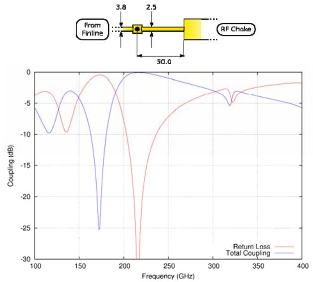
Fig. 15. (Top) Diagram of the single junction tuning circuit. Dimensions are in microns and the SIS junction is shown as a black circle. (Bottom) SuperMix calculated scattering parameters for the single-junction tuning circuit.
