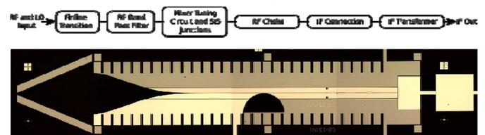
Fig. 11. (Top) circuit components making up the ultra-wide IF band finline SIS mixer. (Bottom) photo of an ultra-wide IF band finline SIS mixer chip prior to dicing and mounting in the mixer block. Apart from the finline taper, left, and the IF bond pads, right, the circuit components are too narrow to be seen in the photo.
