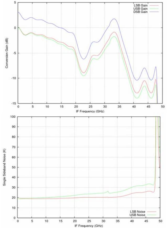
Fig. 24. SuperMix calculated mixer conversion gain (top) and noise temperature (bottom) against IF frequency for the complete single-junction mixer. The mixer is biased at 2.2 mV, and pumped by 100 nW of LO power at a frequency of 220 GHz.
