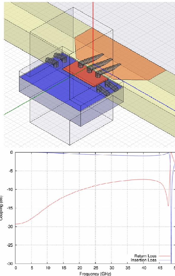
Fig. 18. (Top) HFSS model of the IF bond pads (blue and red), bond wires (grey) and IF output microstrip (pink). Three bond wires connect the mixer wiring to the IF output, while two wires are used on each side to ground the chip to the mixer block. (Bottom) HFSS calculated scattering parameters of the IF connection, normalised to the mixer output impedance of 16.5  $\Omega$ .
