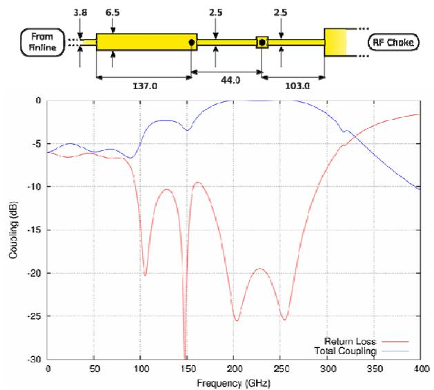
Fig. 16. (Top) Diagram of the dual junction tuning circuit. Dimensions are in microns and the SIS junctions are shown as black circles. (Bottom) SuperMix calculated scattering parameters for the dual-junction tuning circuit.
