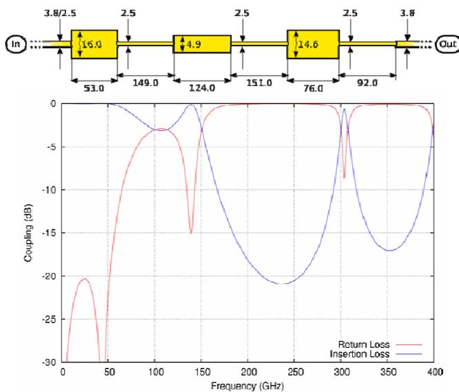
Fig. 17. (Top) Diagram of the stepped width microstrip RF choke. Dimensions are in microns. (Bottom) Sonnet *em* calculated performance of the RF choke.
