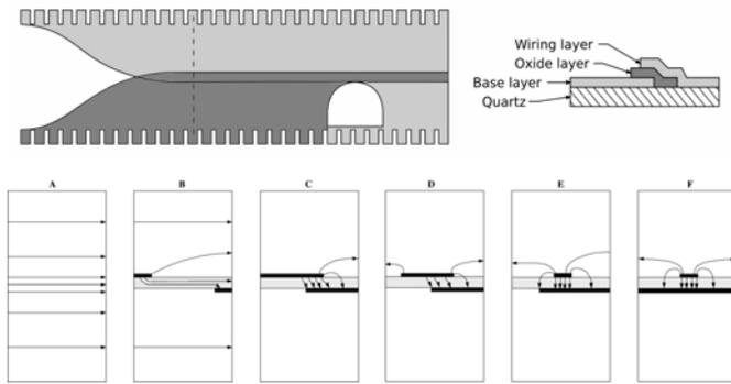
Fig. 12. (Top) Schematic of the modified antipodal finline taper used on these mixers. (Bottom) Cross-sections through an antipodal finline transition, showing E-field lines. **A** Loaded waveguide. **B** Unilateral finline section. **C** Antipodal finline section. **D** 1<sup>st</sup> half of circular finline to microstrip transition. **E** 2<sup>nd</sup> half of circular finline to microstrip transition. **F** Output microstrip.
