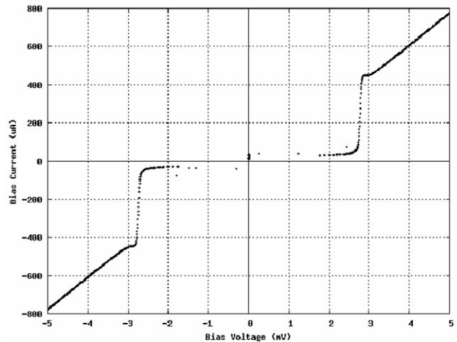
Fig. 20. Measured I-V curves for a dual-junction mixer from the first fabrication batch.
