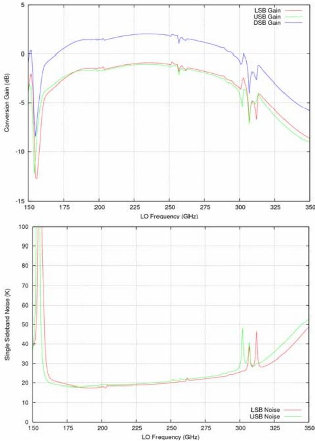
Fig. 23. SuperMix calculated mixer conversion gain (top) and noise temperature (bottom) against LO frequency for the complete single-junction mixer. The mixer is biased at a fixed bias voltage of 2.2 mV, and pumped with a fixed LO power of 100 nW. The IF frequency is 5 GHz. The narrow spikes in the performance just above 250 and 300 GHz are artefacts caused by running the simulation at a fixed bias voltage and LO power.
