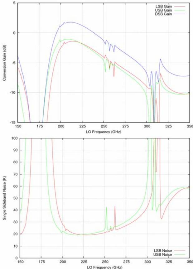
Fig. 21. SuperMix calculated mixer conversion gain (top) and noise temperature (bottom) against LO frequency for the complete single-junction mixer. The mixer is biased at a fixed bias voltage of 2.2 mV, and pumped with a fixed LO power of 50 nW. The IF frequency is 5 GHz. The narrow spikes in the performance just above 250 GHz and 300 GHz are artefacts caused by running the simulation at a fixed bias voltage and LO power.
