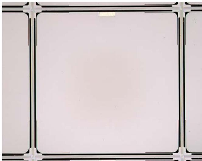
Figure 3. This micrograph of a single pixel shows the style of thermal attachment to the beams making up the bolometer array grid. The TES is the small gold rectangle at the top edge
